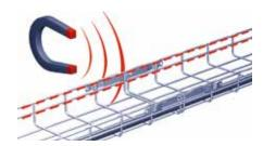
• Connect the cable trays to the bonding system (every 15 to 20 m)
