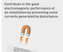
The metal structure of the cable tray absorbs some of the electromagnetic disturbance and converts it into noise current.
