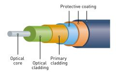
The optical cladding confines the optical waves in the core: the light ray is propagated by successive reflections on the walls formed by the optical cladding. The protective coating, usually a layer of plastic of 25 to 1000 microns, confers the fibre with remarkable mechanical properties.
